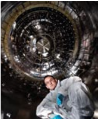
Figure 3. Jasper Kirkby inside the 3.5-meter-(~10.5-foot)-diameter chamber used for CLOUD (Cosmics Leaving OUTdoor Droplets) experiments. Image: CERN.
