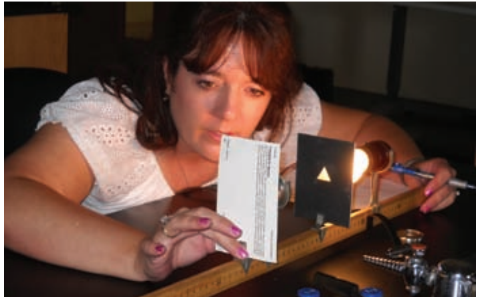
An ICR graduate student measures the focal length of a lens during a laboratory lesson.
