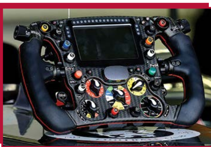
Figure 1. The Sauber C33 is a typical Formula 1 steering wheel. While traveling over 200 mph, the driver manages this jam-packed steering wheel housing, his gear-shift paddles, communications toggles, and 16 buttons and nine rotary switches—all sending vehicle information. This steering wheel costs in the neighborhood of $40,000.
